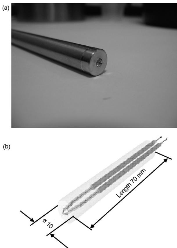
Fig. 1. Appearance (a) and design (b) of fibre probe tip with ATR cone element.
