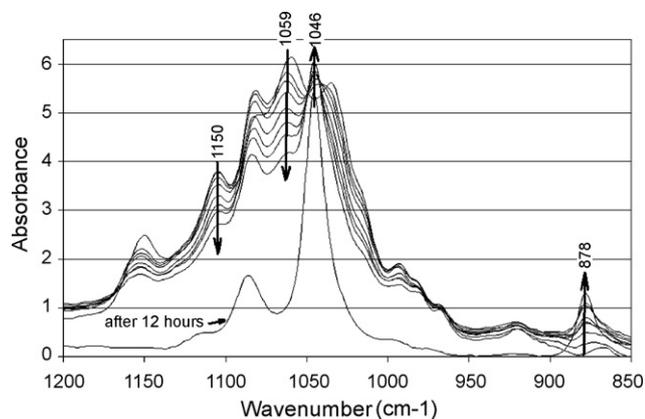
**Fig. 6.** Absorption spectra of chemical reaction mixture of alcohol fermentation as function of time (measurements carried out every 60 min): absorption bands of ethyl alcohol (increasing) and sugar (decreasing).
