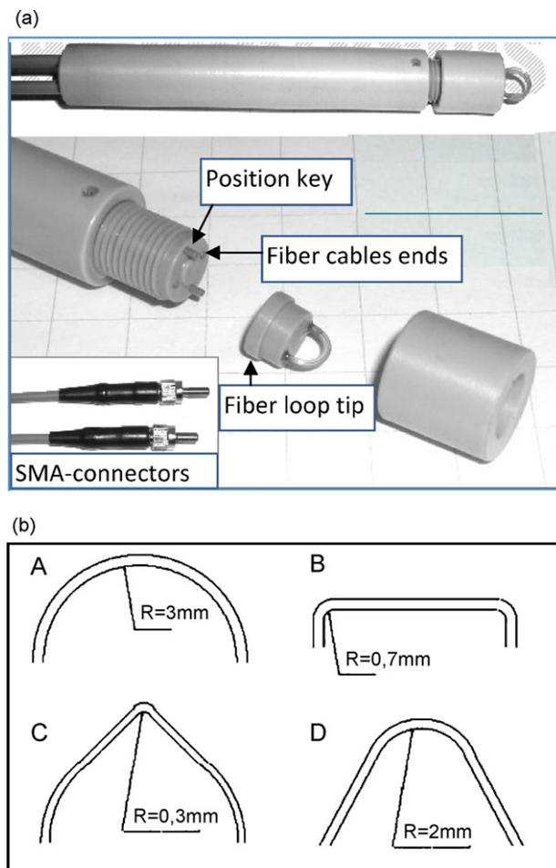
Fig. 2. Appearance and design of fibre probe tip with detachable loop ATR element (a). Disposable fibre loops of different shape (b): standard U-shaped (A), “rectangle” (B), “triangle” (C) and V-shaped (D).
