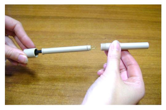
Screw on and tighten the screw nut. Rotate the nut but not the cap.
