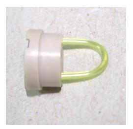
Prevent any contamination of the fibre ends on the probe tip. Take care not to lose Teflon sealing ring (inside the fixing cap).
