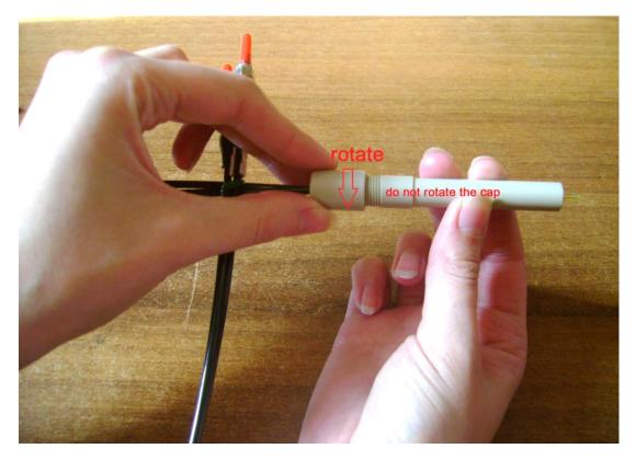
Take the old loop from the slot on the probe and prepare a new loop tip.
