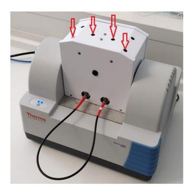
Delete small plugs from the holes with tuning screws.
