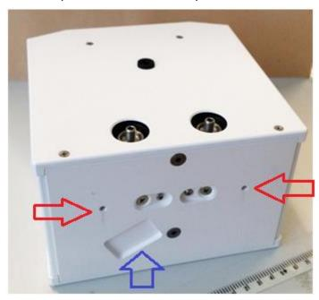
Holes for positioning pins are shown with red arrows, the groove for the electronic chip is shown with blue.
