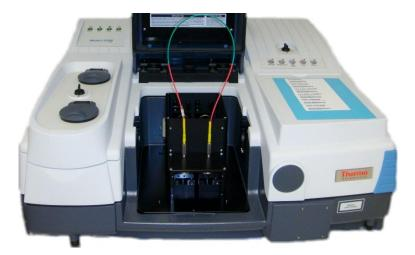
The preparation is ready for the alignment of fiber probe coupler to get highest signal possible.
