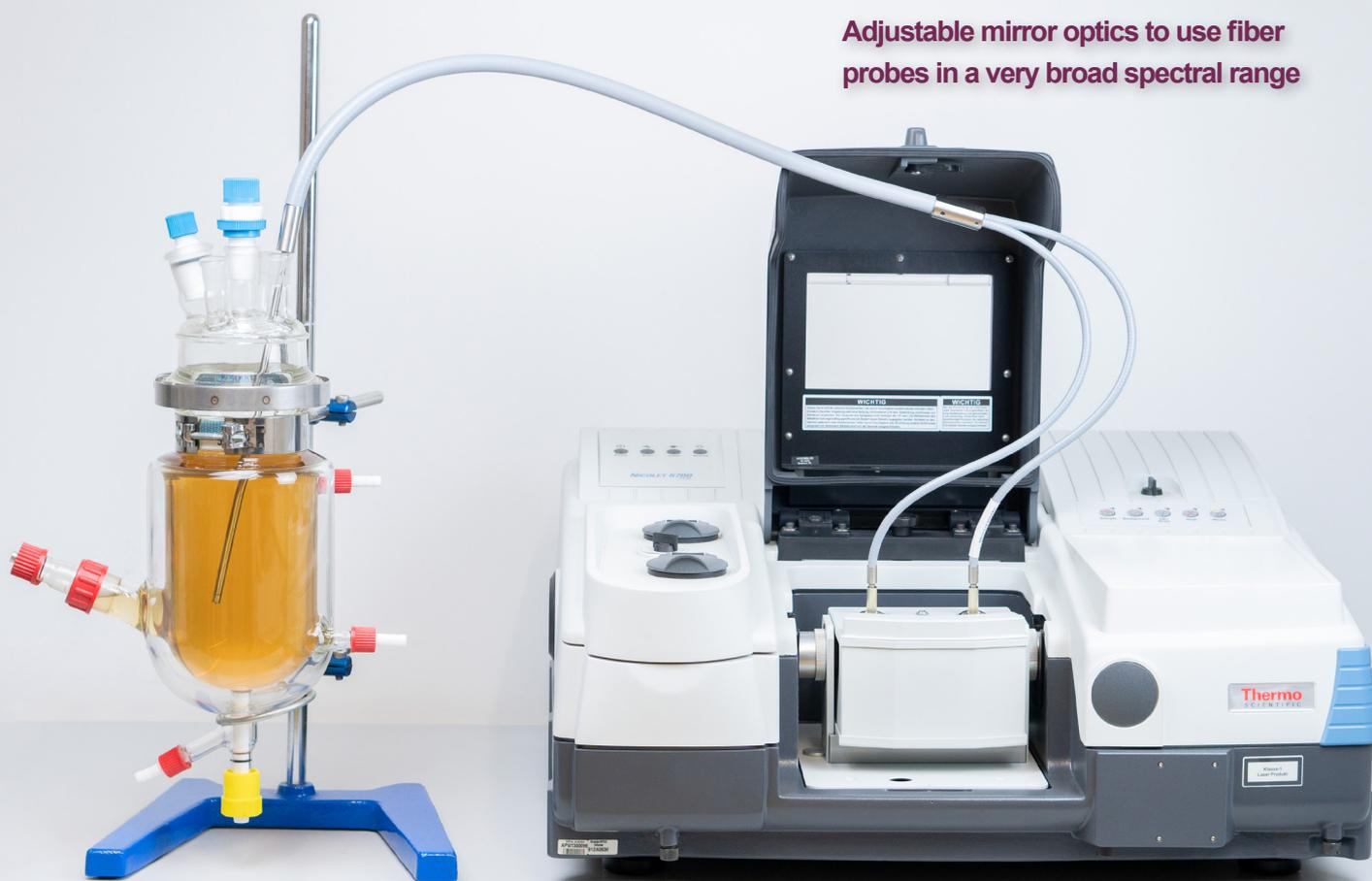
**Fiber Probe Couplers** enable coupling of *FlexiSpec*® fiber probes with any FTIR-spectrometer when installed in its sample chamber. Various *FlexiSpec*® probes can be used for remote media analysis in-citu & in real time - for reaction monitoring and process control – instead of time consuming samples collection & preparation. Mirror design of *FlexiSpec*® **Fiber Probe Couplers** provides high coupling efficiency for any probe used for process-spectroscopy in broad spectral range 0.2-18µm.
